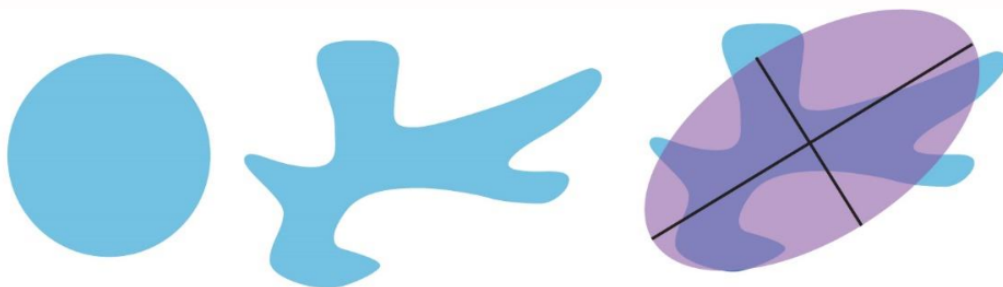
Figure 56: Left: a circle is the most compact shape, with a compactness of 1. Middle: a shape whose compactness is less than 1. Right: the eccentricity of the shape is computed as the eccentricity of the best-fitting ellipse.
