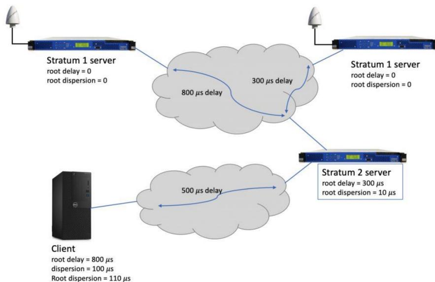
Figure 9: Example root dispersion & root delay
