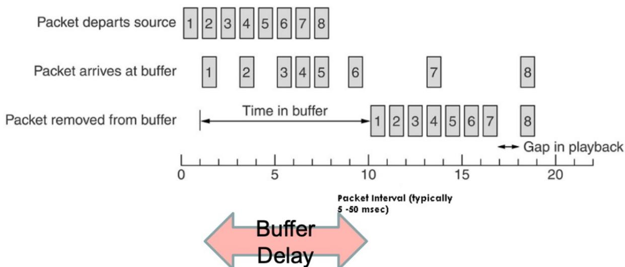
Figure 19: Receiver-based packet loss strategies: jitter buffer strategies
