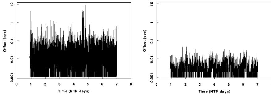
Figure 12: Clock filter algorithm before and after
