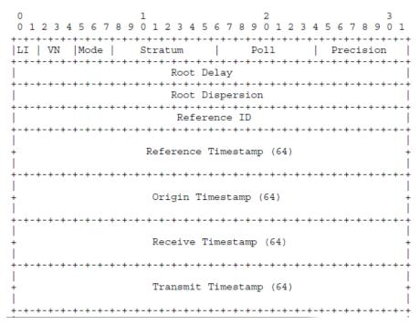
Figure 8: NTP protocol header
