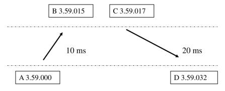
Figure 7: Network delay asymmetry
