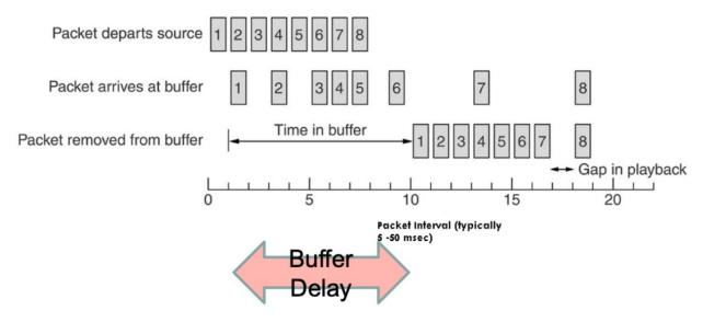
Figure 19: Receiver-based packet loss strategies: jitter buffer strategies
