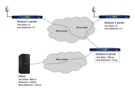
Figure 9: Example root dispersion & root delay
