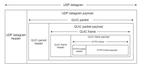
Figure 34: QUIC packet structure
