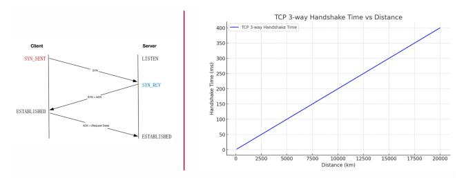
Figure 25: The TCP 3-way handshake is expensive
