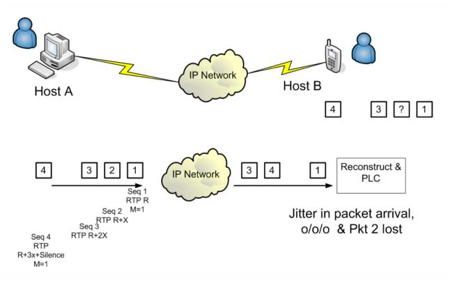
Figure 17: RTP data delivery
