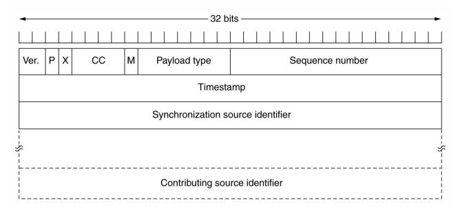
Figure 16: RTP header
