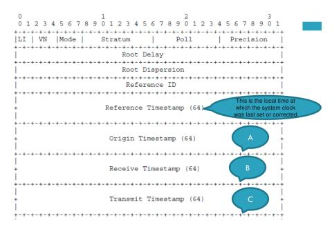
Figure 10: Annotated NTP protocol header
