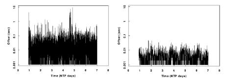
Figure 12: Clock filter algorithm before and after
