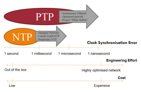
Figure 3: NTP & PTP characteristics
