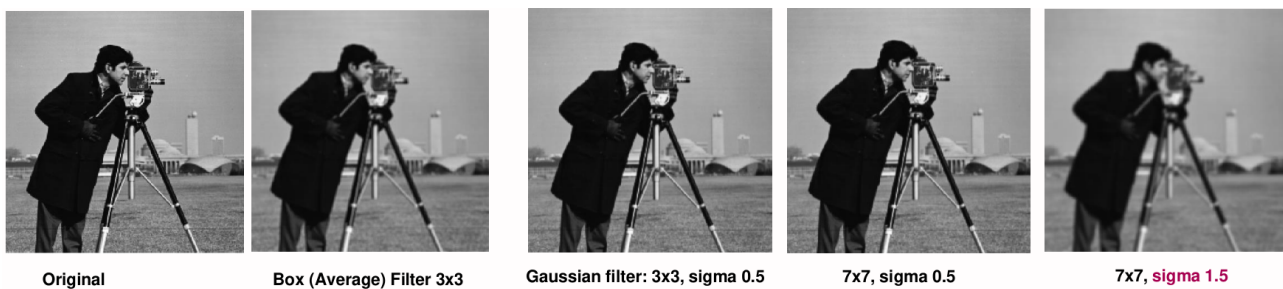
Figure 29: Spatial Filtering: Smoothing Filters
