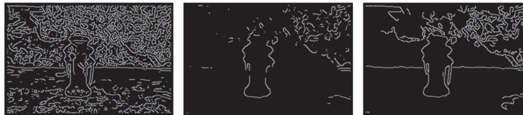
Figure 67: Edge linking with hysteresis, also known as double thresholding or hysteresis thresholding. Thresholding the gradient magnitude with the low threshold produces too many edge pixels (left), while thresholding the high threshold produces too few edge pixels (middle). Edge linking with hysteresis combines the benefits of both (right) to produce the final Canny edge detector output.
