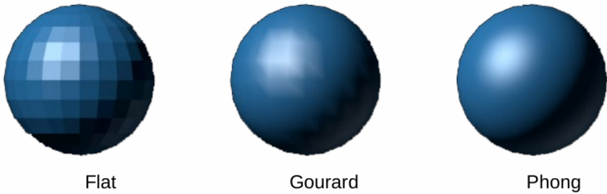
Figure 16: Different Shading Algorithms
