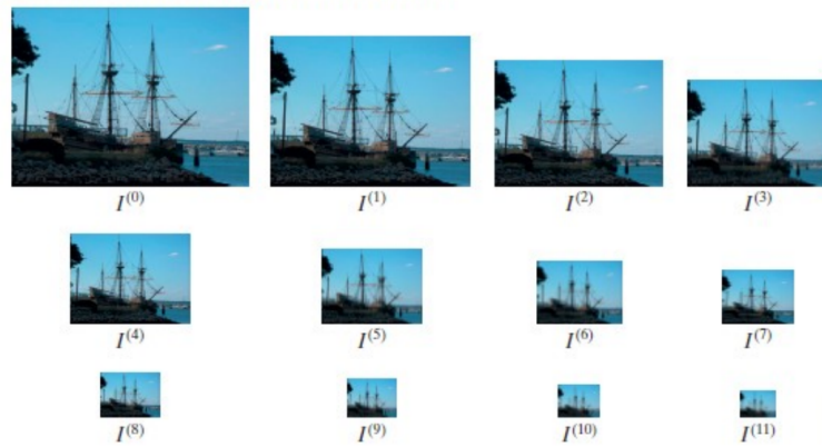
Figure 61: Twelve levels of a Gaussian pyramid, obtained with \sigma^2 = \frac{1}{4}(0.5) = 0.125 and a downsampling factor of \sqrt[4]{2} . Note that I^{(4)} is half as large as I^{(0)} in each direction, and that I^{(8)} is half as large as I^{(4)} .
