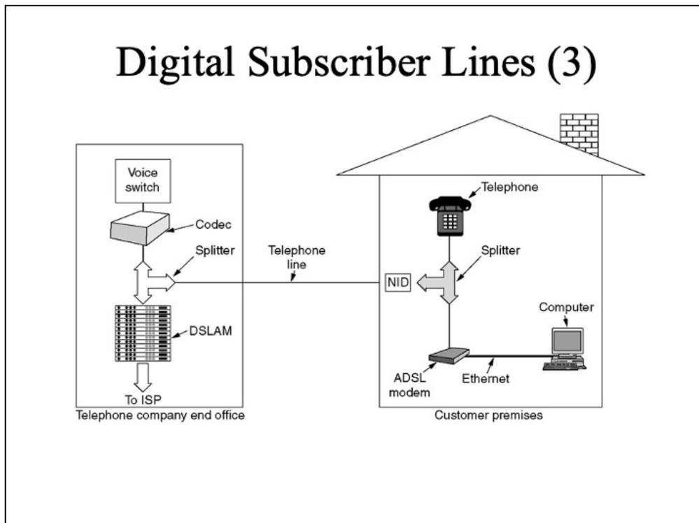
A telephone company technician must install a NID (NETWORK INTERFACE DEVICE) in the customer's house. Close or combined with the NID, a SPLITTER is installed, which is an analog filter that separates the phone signal (0 to 4000Hz) from the data signal (over 26kHz).
