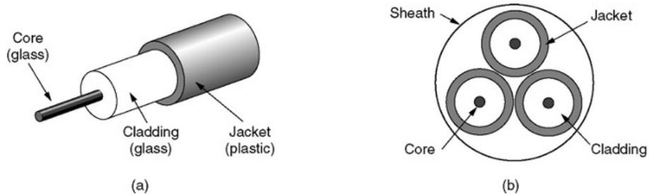
Multimode fibers, the core is 50 microns. For single mode fibers, the diameter of the core is 8 to maximum 10 microns.
