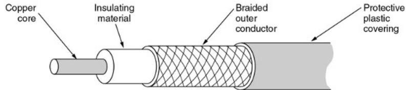
It is better shielded than twisted pair cable and it can span over longer distances at higher speeds. 50 ohms (for digital transmission) and 75 ohms (for analog transmission) are available. Due to the construction and the shielding process, the coax cables can have large bandwidth (up to 1GHz). They used to be largely used by phone companies for long distance lines, but now they have been replaced with fiber optics.
