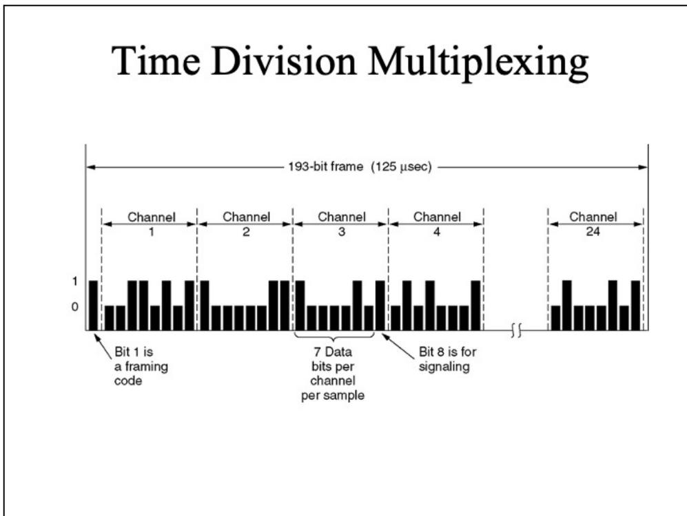
How multiple analog voice telephone channels are digitized and combined onto a single outgoing digital trunk.
