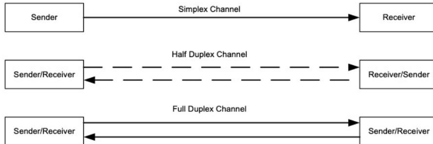
The message source is the transmitter, and the destination is the receiver. A channel whose direction of transmission is unchanging is referred to as a simplex channel. For example, a radio station is a simplex channel because it always transmits the signal to its listeners and never allows them to transmit back.
