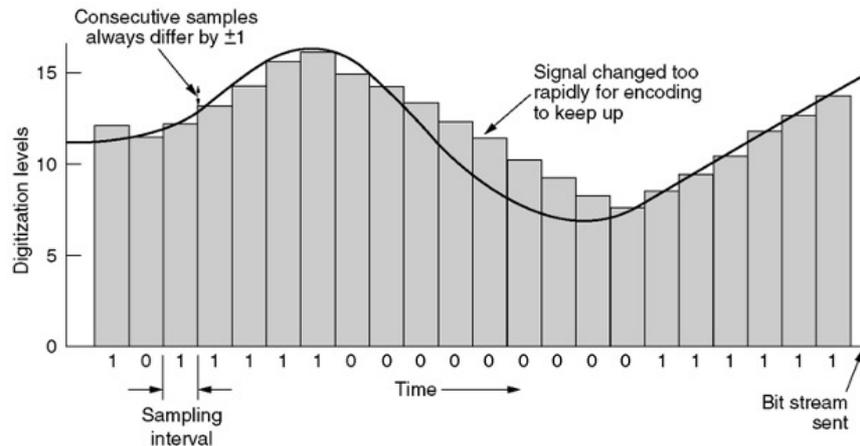
Once the voice channel has been digitized, it is tempting to use statistical techniques to obtain fewer bits per sample (therefore lower bandwidth required to carry the voice information). All the compaction methods are based on the fact that the analog voice signal is changing relatively **SLOWLY** compared to the sampling frequency, so much in the information in the 7<sup>th</sup> and 8<sup>th</sup> bit is redundant.
