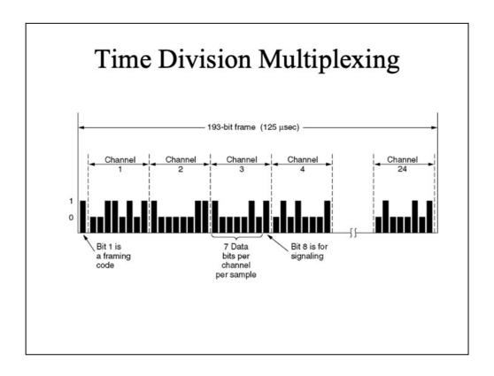
How multiple analog voice telephone channels are digitized and combined onto a single outgoing digital trunk.
