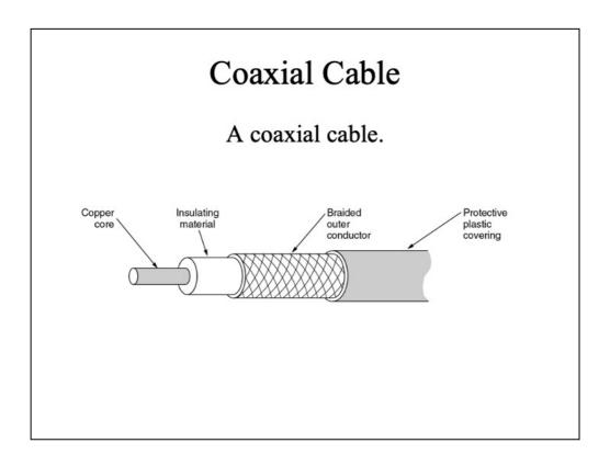
It is better shielded than twisted pair cable and it can span over longer distances at higher speeds. 50 ohms (for digital transmission) and 75 ohms (for analog transmission) are available. Due to the construction and the shielding process, the coax cables can have large bandwidth (up to 1GHz). They used to be largely used by phone companies for long distance lines, but now they have been replaced with fiber optics.
