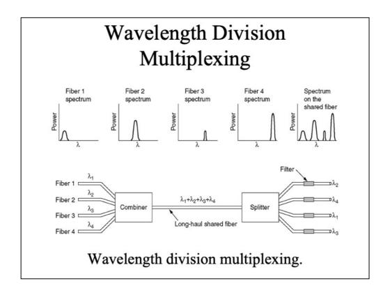
It is a variation of the FDM at very high frequencies and it is used over the optical fiber trunks. Systems with 96 channels of 10Gbps each are available in production. 960 Gbps is enough to send 30 full time movies per second...
