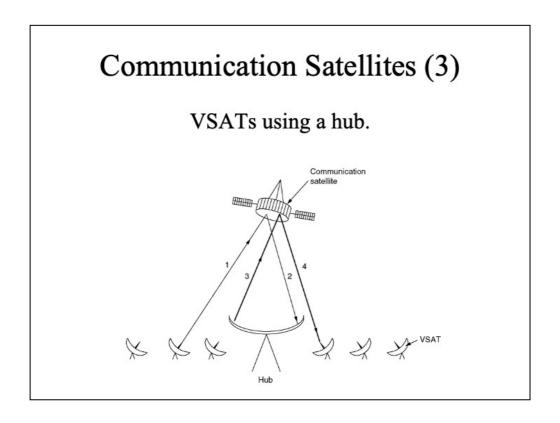
VSAT – VERY SMALL APPERTURE TERMINALS – 1 meter or smaller compared to 10 meters required for GEO satellites communication.
