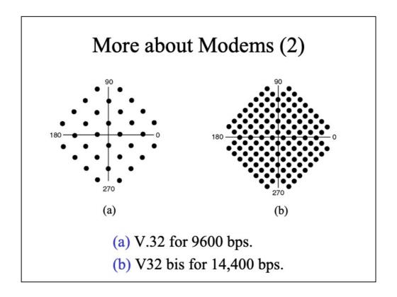
With many points in the constellation diagram, even a small amount of noise would result in transmission errors.
