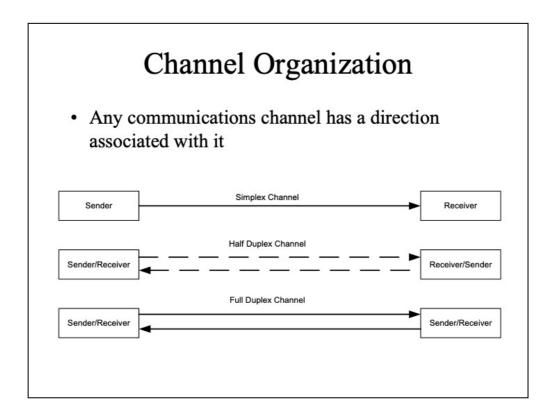
The message source is the transmitter, and the destination is the receiver. A channel whose direction of transmission is unchanging is referred to as a simplex channel. For example, a radio station is a simplex channel because it always transmits the signal to its listeners and never allows them to transmit back.
