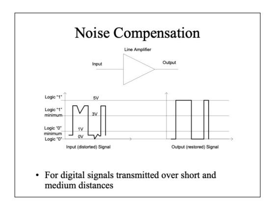
These effects are properties of transmission through metallic conductors, and become more pronounced as the conductor length increases. To compensate for distortion, signal power must be increased or the transmission rate decreased.
