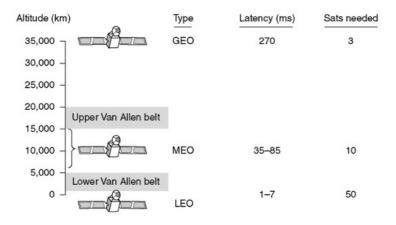
Communication satellites and some of their properties, including altitude above the earth, round-trip delay time and number of satellites needed for global coverage.
