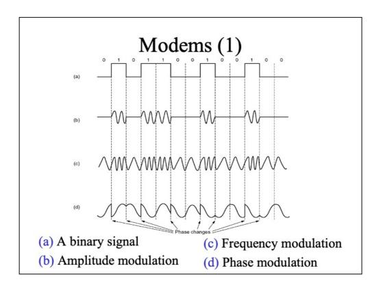
A modem is a device that accepts a serial stream of bits as input and produces a carrier modulated by one (or more) of these methods (modulator/demodulator). The modem is inserted between the (digital) computer and the (analog) telephone system.
