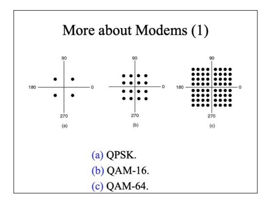
QPSK – QUADRATURE PHASE SHIFT KEYING – four phases are used
