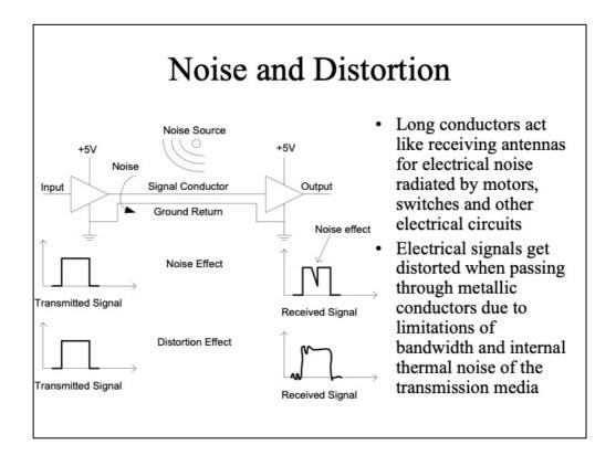
Because of the very high switching rate and relatively low signal strength found on data, address, and other buses within a computer, direct extension of the buses beyond the boudaries of the main circuit board or plug-in boards would pose serious problems.
