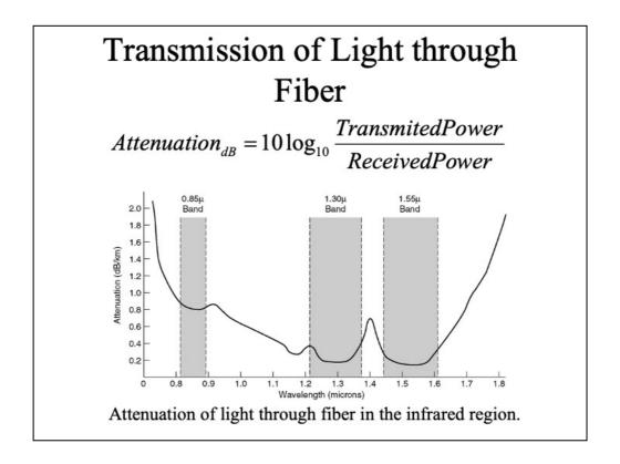
The attenuation of light through glass (the raw material used for optical fiber cable) depends on the wavelength of the light but also on the physical properties of the glass.
