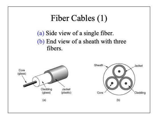
Multimode fibers, the core is 50 microns. For single mode fibers, the diameter of the core is 8 to maximum 10 microns.
