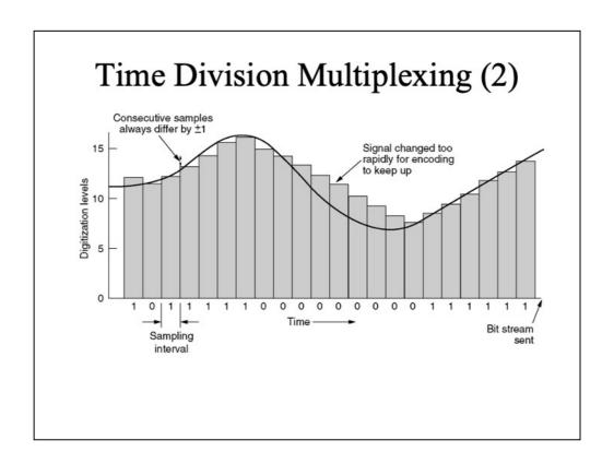
Once the voice channel has been digitized, it is tempting to use statistical techniques to obtain fewer bits per sample (therefore lower bandwidth required to carry the voice information). All the compaction methods are based on the fact that the analog voice signal is changing relatively **SLOWLY** compared to the sampling frequency, so much in the information in the 7<sup>th</sup> and 8<sup>th</sup> bit is redundant.
