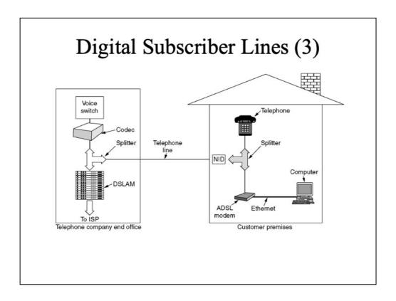
A telephone company technician must install a NID (NETWORK INTERFACE DEVICE) in the customer's house. Close or combined with the NID, a SPLITER is installed, which is an analog filter that separates the phone signal (0 to 4000Hz) from the data signal (over 26kHz).
