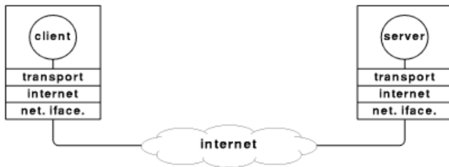
Figure 1: Client & server using TCP/IP protocols to communicate. Information can flow in either or both directions. The client & server can interact with a transport layer protocols.
