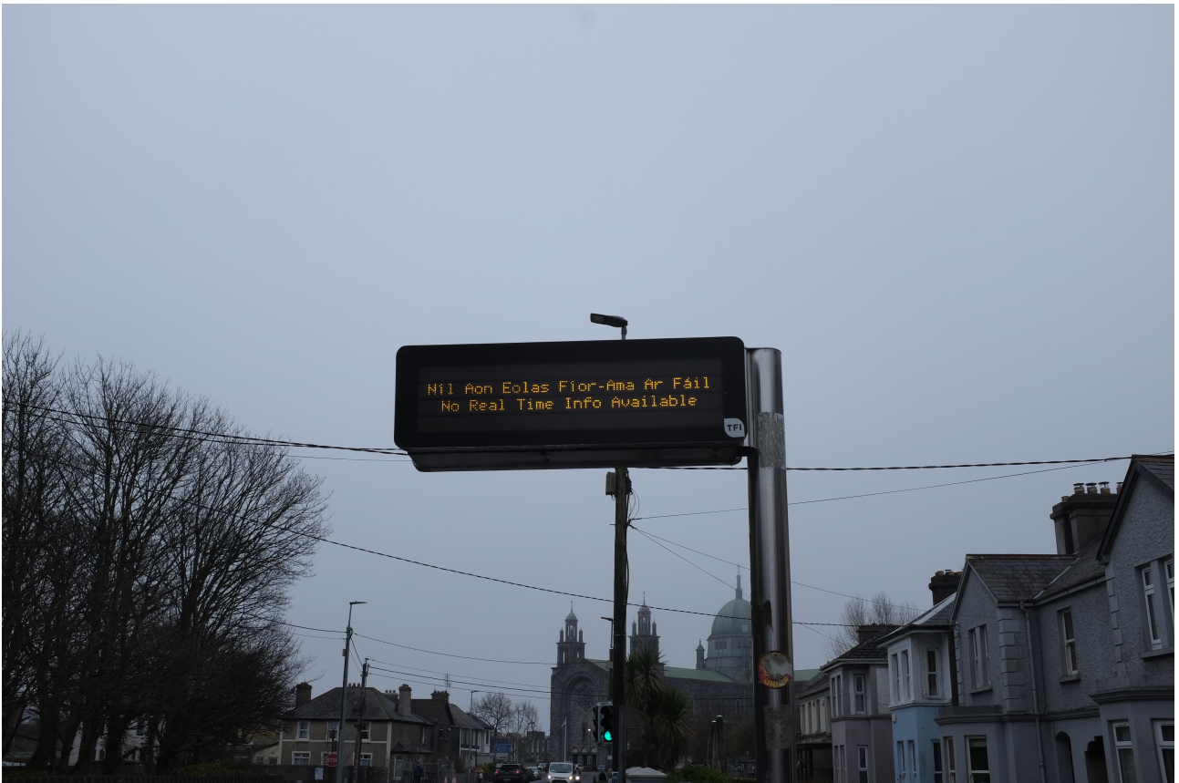
Figure 1.1: Photograph of the University Road Bus Éireann information display erroring due to the clocks going back [2025-03-30]
