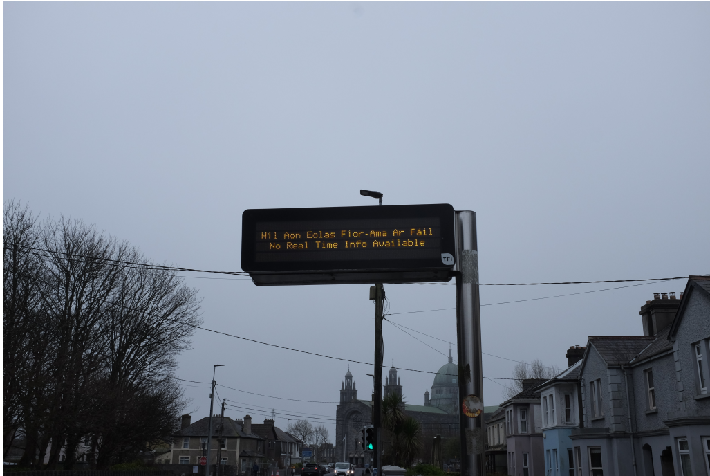
Figure 1.2: Photograph of a TFI display erroring due to the clocks going forward [Taken: 2025-03-30]
